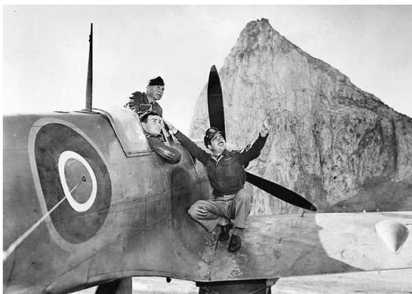
**The wire IFF antenna and VHF radio antenna can be clearly seen on this Spitfire Mark Vb. The insulator for the IFF wire to the tailplane can be seen on the centre part of the fuselage roundel.**
