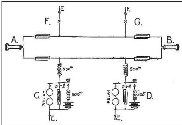
**Figure 2 - The Van Rysselberghe Circuit (Note: The C and D circuit is duplicated at F and G).**
