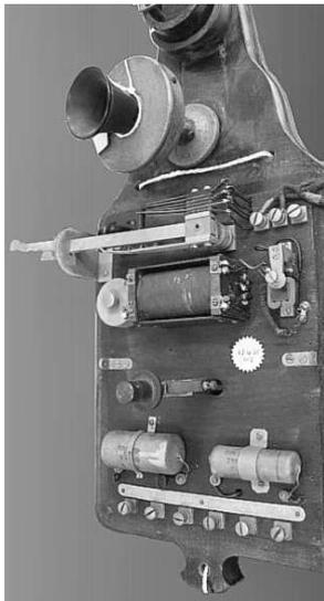
**Figure 4 - Phonopore with front cover removed.**
