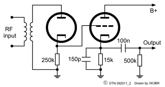
actually slightly higher as well! I don't know if the circuit, Fig 1, is completely optimised, but it certainly works well and produces great sounding audio from AM broadcasting stations!
